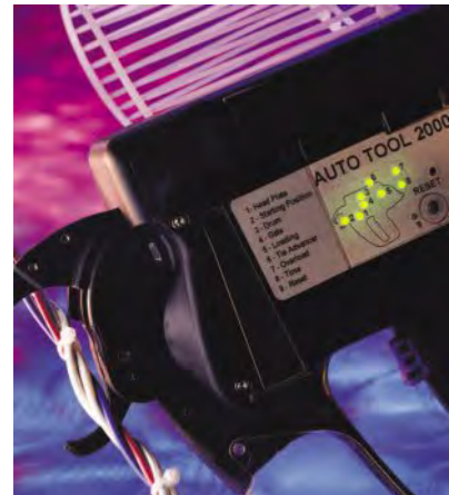
An LED panel shows the status of the tool.
