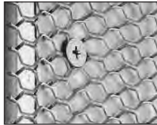
Wire lath to steel or wood studs.
