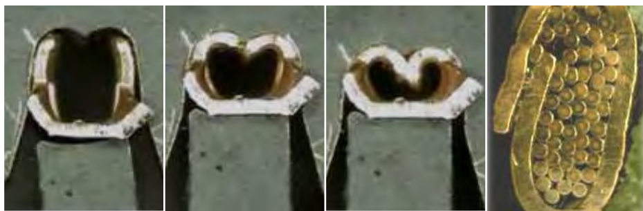
Rolling-in of crimp area is not uniform
