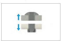
This is the force the rivet can stand in the direction to its longitudinal axis when strained until the rivet joint breaks down.
