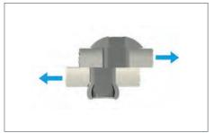
This is the force, acting horizontally to the longitudinal axis, the rivet can stand when strained until the rivet joint breaks down.
