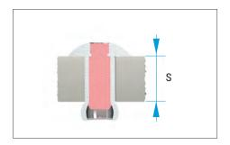
The material thickness has to be within both, the minimal and maximal value the rivet is constructed for.
