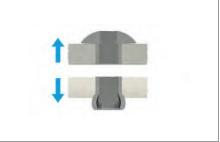
This is the force the rivet can stand in the direction to its longitudinal axis when strained until the rivet joint breaks down.
