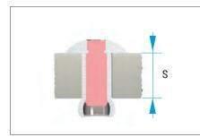
The material thickness has to be within both, the minimal and maximal value the rivet is constructed for.
