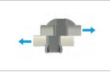
This is the force, acting horizontally to the longitudinal axis, the rivet can stand when strained until the rivet joint breaks down. This force is stated in N=Newton. This test is standardised according to DIN EN ISO 14598. Tensile Strength
