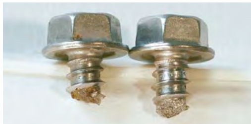
Example of how fasteners can fail due to hydrogen-assisted cracking (HAASC). These 410 SS super passivated fasteners with plain finish (above) and 410 fasteners with aluminum-filled topcoat (below) failed at the interface of the aluminum and steel sheets during salt spray tests.
