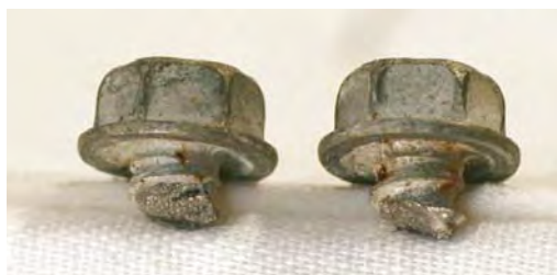
Example of how fasteners can fail due to hydrogen-assisted cracking (HAASC). These 410 SS super passivated fasteners with plain finish (above) and 410 fasteners with aluminum-filled topcoat (below) failed at the interface of the aluminum and steel sheets during salt spray tests.
