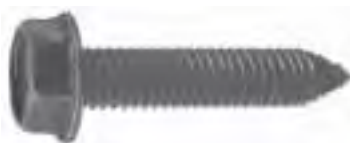
12009 Phosphate & Oil 5/16"-18 x 1-1/2" Hex Washer Head 21/32" Washer Head O.D. 1/2" Hex GM
