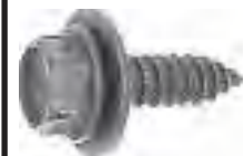
12351 (11505022) Black Polyseal Finish M6.3-1.81 x 20mm (#14 x 25/32") Hex Washer Head Sems® 17mm (11/16") Wshr O.D. 10mm Hex GM
