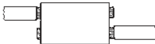
Parallel Connectors Proper Wire Insertion
