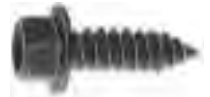
13019 (N610959-S2) Phosphate M6.3-1.81 x 19mm (#14 x 3/4") Hex Washer Head 11.5mm (29/64") Washer Hd. O.D. 8mm Hex Ford
