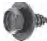
12057 (11500994, 11509371) Phosphate M6.3-1.81 x 16mm (#14 x 41/64") Hex Head Sems® 17mm (11/16") Wshr O.D. 10mm Hex GM
