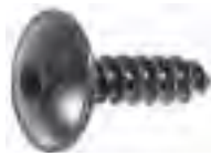
21541 (13144822) Black Zinc M5.5 x 20mm (12 x 25/32") Torx® Truss Head T-20 Drive 15mm (19/32") Head O.D. Use With Auveco 21539 & 21540 GM 2011 - On Saab 2003 - On
