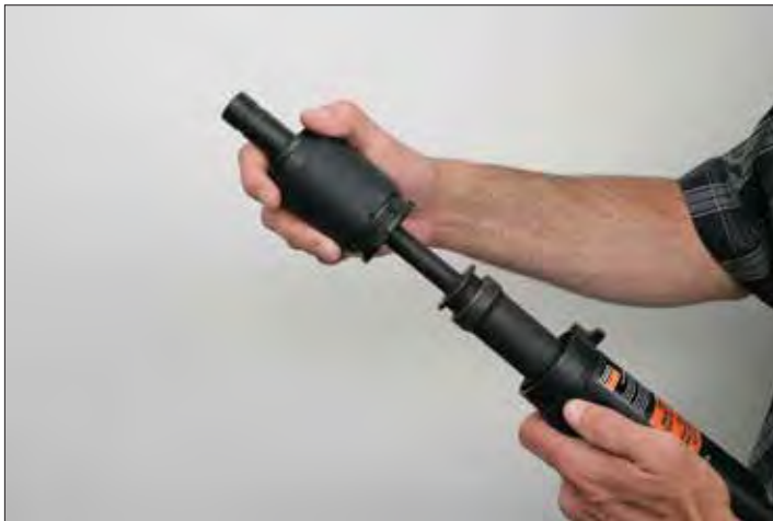
Quick-disconnect baseplate makes it easy to convert the PTP-27SMAGR from a magazine to a single-shot tool.
