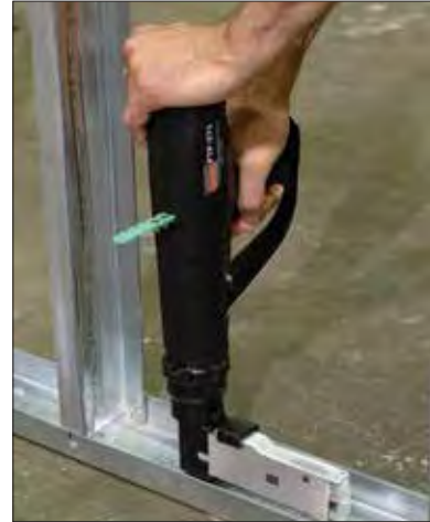
Rotating magazine allows for installation flexibility.
