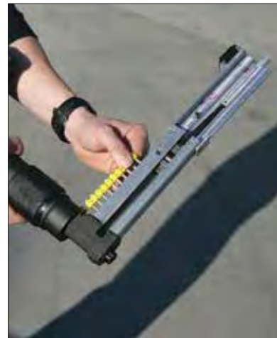
Collated pins make for fully automatic fastening and quick loading.
