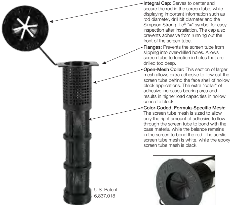
Epoxy Adhesive Screen Tube (mesh is black)
