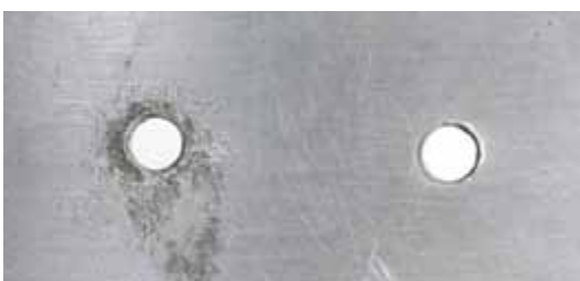
The modified 400 SS fasteners, 410 SS super passivated fasteners with plain finish, and 410 fasteners with aluminum-filled topcoat failed at the interface of the aluminum and steel or directly under the fastener head.
