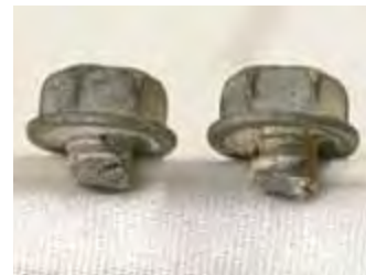
The modified 400 SS fasteners, 410 SS super passivated fasteners with plain finish, and 410 fasteners with aluminum-filled topcoat failed at the interface of the aluminum and steel or directly under the fastener head.
