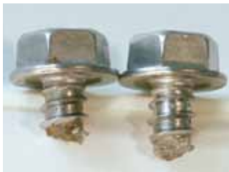
The modified 400 SS fasteners, 410 SS super passivated fasteners with plain finish, and 410 fasteners with aluminum-filled topcoat failed at the interface of the aluminum and steel or directly under the fastener head.
