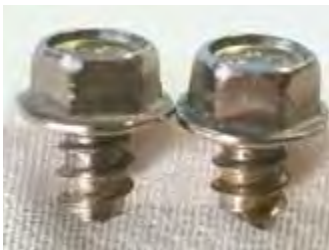
The modified 400 SS fasteners, 410 SS super passivated fasteners with plain finish, and 410 fasteners with aluminum-filled topcoat failed at the interface of the aluminum and steel or directly under the fastener head.
