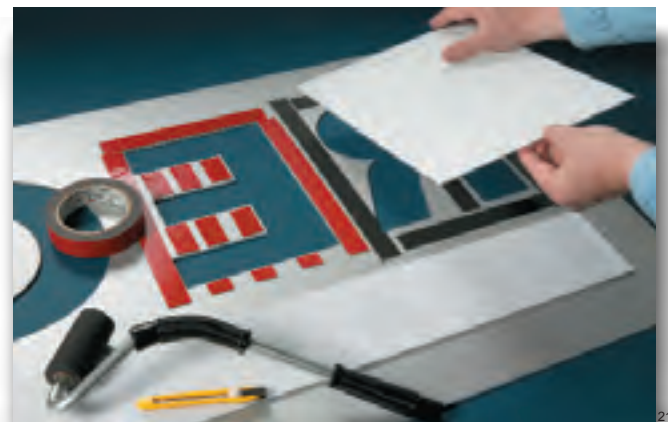
Easily cut to size, 3M™ VHB™ Tape 5952 bonds polycarbonate sheets to the back of a routed aluminum face. Surface is simply cleaned prior to application. Tape is pressed with a roller for optimum bonding.
