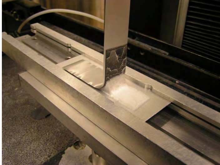
Ninety degree peel adhesion testing showing “adhesive split” of 4412N tape. (Black area is 5925 tape bonding the aluminum foil peel strip to non-adhesive, ionomer film side of 4412N.)
